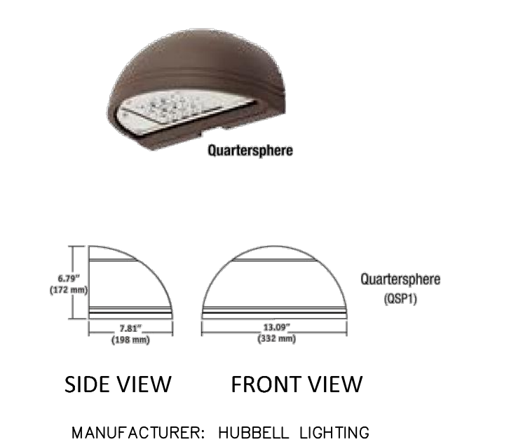
4 WALL-MOUNTED LIGHT FIXTURE DETAIL SCALE: NTS
