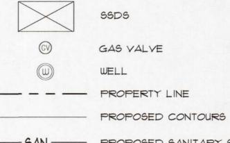
== SAN === PROPOSED SANITARY SEWER LINE EXISTING SMH PROPOSED SANITARY SEWER MANHOLE
